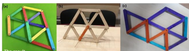
Figure 3. Actual truss designed by students
