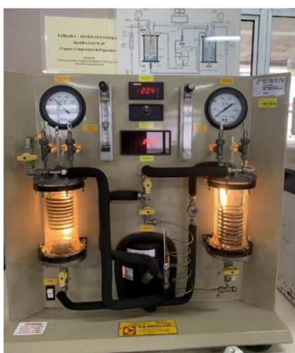
Figure 6: Lab refrigeration system in operation
